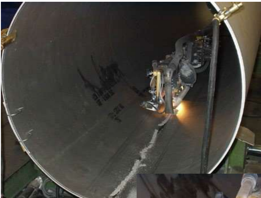
Versatile flux for welding stainless steels, but also suitable for welding Ni-alloys as well as low alloyed steels.
