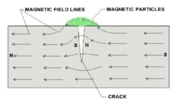
The first step in a magnetic particle inspection is to magnetize the component that is to be inspected. If any defects on or near the surface are present, the defects will create a leakage field. After the component has been magnetized, iron particles, either in a dry or wet suspended form, are applied to the surface of the magnetized part. The particles will be attracted and cluster at the flux leakage fields, thus forming a visible indication that the inspector can detect.
