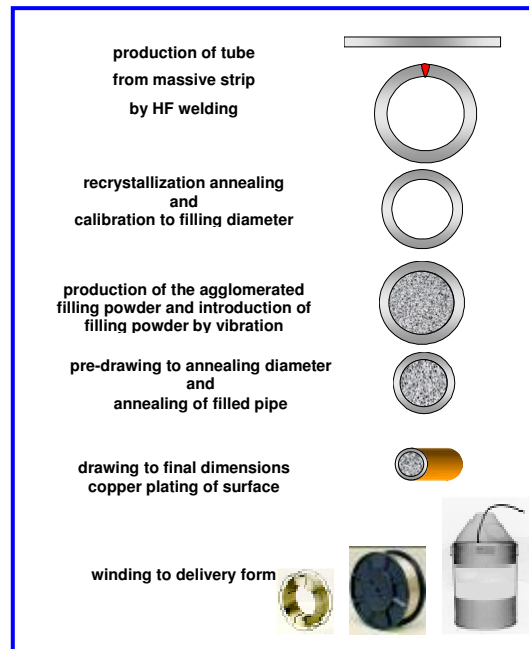
figure 3: production of STEIN-MEGAFIL flux-cored wires
