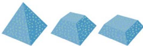
The three-dimensional structures of 3M™ Trizact™ Abrasives contain multiple layers of mineral. As these structures wear, fresh, sharp mineral is constantly exposed to the workpiece, resulting in faster, more consistent cutting throughout the life of the belt.
