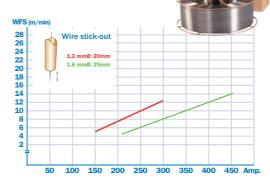
\* The above values and parameters are for all weld metal produced using 100%CO<sub>2</sub> shielding gas
