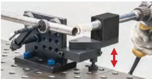
Notch 25 – 63.5 mm OD pipes or square tubes at any angle, or off-center. Position the two V-Blocks and clamp as needed.
