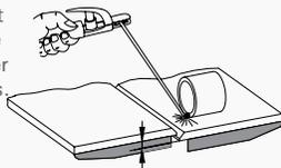
Slide Half Clamp onto the cut pipe, turn the handle until the misaligned materials align.
