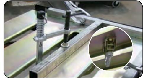
The MagSpring™ Clamps can be inserted into the 28 mm slots on the Nomad™ Tabletop for hold down clamping. Magnetic V-Pad jaw holds underneath the table to keep the clamp in the up-right, "ready to use" position.
