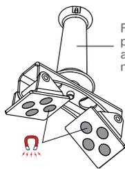
For control in placing, positioning and breaking the magnetic force.
